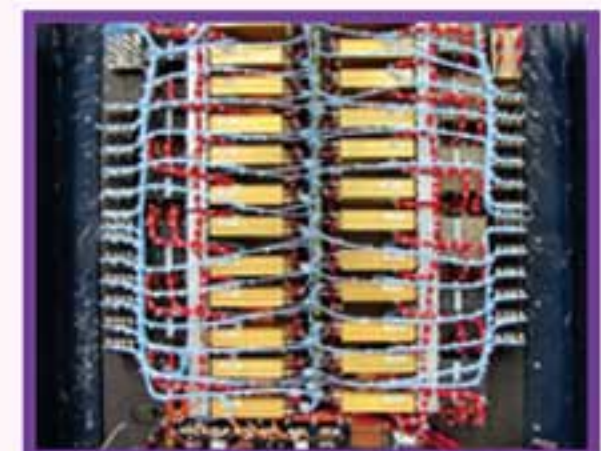
RISAT-1A: DVM Tile electronics
