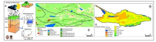
Fig. 2: a): Schematie of VIC Hydrological Model; b) LULC of the IIe River Basin (Source: Copernicus); e) Soil Texture of the IIe River Basin (Source: FAO)
