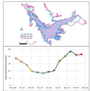
**Fig.1:** (a) Spatial and (b) temporal variation of surface water spread (12/2020 – 12/2021) for Ramganga reservoir
