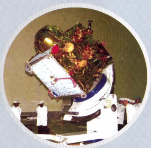
IRNSS-1A undergoing tests in clean room
